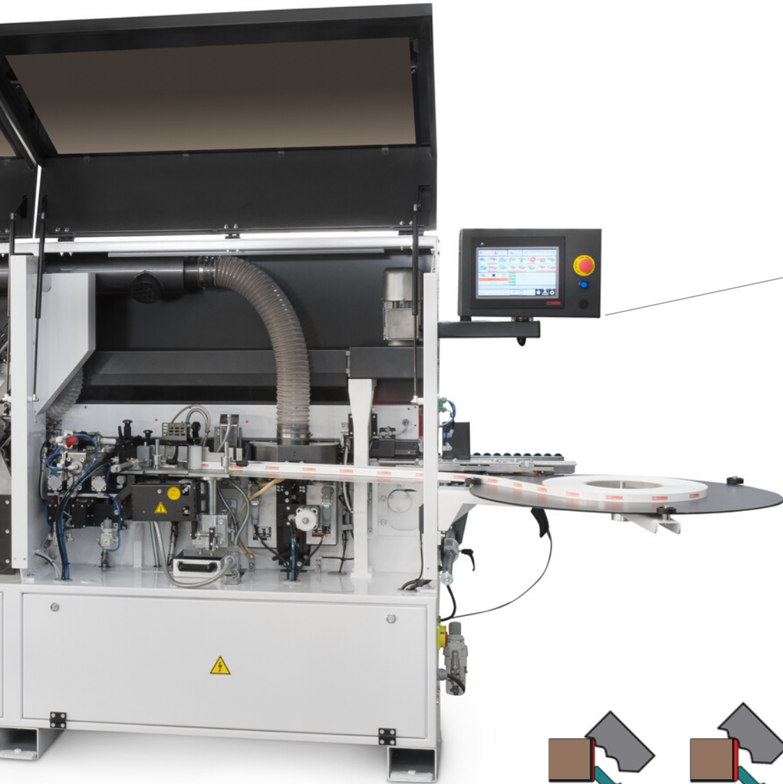
Multi-profile motor driven T&B Trim and Radius Scraper units
